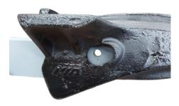
**STEP ONE** Slide the ripper point onto the shank, lining up the bolt holes.
