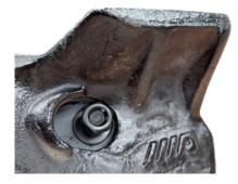
**STEP THREE** Ensure that a washer is present on each end of the bolt and fasten securely with a nut, retaining the ripper point onto the shank.
