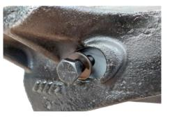
**STEP TWO** Fit the bolt through the lined up holes of the point and shank.
